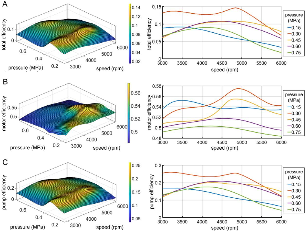
Fig. 6 Our developed mechatronic system achieved relatively high efficiency (A) thanks to the high contributions of motor only (B) and pump only (C). A maximum value of about 15% is recorded at 0.32 MPa and 5000 rpm, which is comparably higher than peak efficiencies reached by other state-of-the-art systems on a similar scale.
